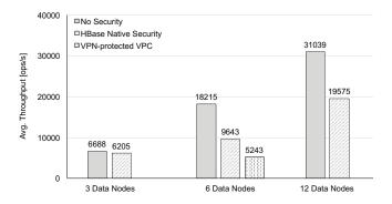
Figure 6. Compared average throughput results for no security, HBase native security, and VPN-protected VPC
