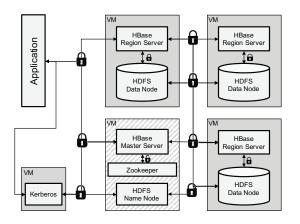
Figure 2. HBase deployment using HBase native security
