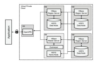
Figure 3. HBase deployment using a VPN-protected virtual private cloud
