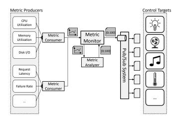
Figure 1. High-Level Architecture of MultiSense
