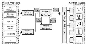
Figure 1: High-Level Architecture of MultiSense
