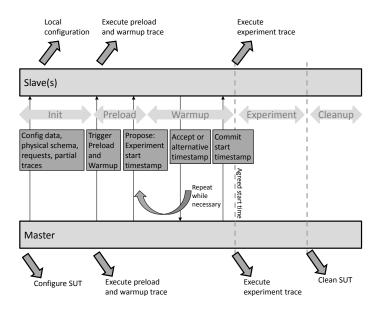
Fig. 2: Execution Phases and Distributed Coordination
