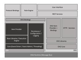
Fig. 1. Overview of the OpenHAB System Architecture. Showing the Eclise SmartHome Core (left) and the OpenHAB specific extensions (right) as well as common modules.
