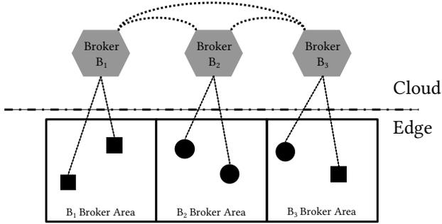
Figure 2: Setup with three brokers that support communication between publishers (squares) and subscribers (circles).
