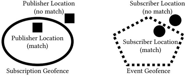
Figure 1: Subscription GeoCheck (left) and event GeoCheck (right), adapted from [7], [8].
