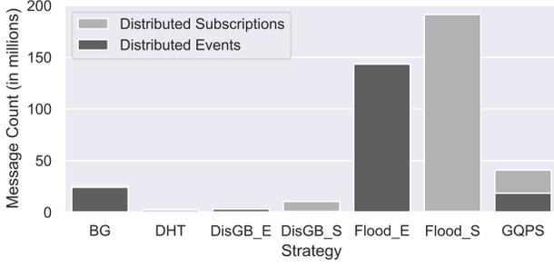
Figure 10: For 100,000 clients and 256 brokers, DHT requires the fewest inter-broker messages.
