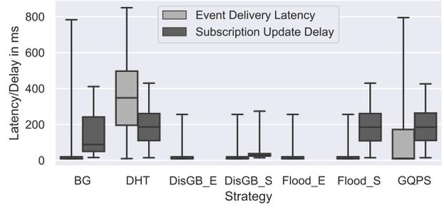
Figure 12: For 100,000 clients and 256 brokers, latency and delay increase slightly compared to Figure 11 as having more brokers increases the likelihood of inter-broker communication.
