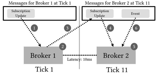
Figure 8: Broker 1 receives a subscription update at Tick 1 (1). Besides updating its state (2), it must distribute the update to Broker 2 as specified by its RP selection strategy (3). As the latency is 10ms, Broker 2 receives the subscription update at Tick 11 (4). It does not need to be further distributed so it is only used to update the broker’s state (5). After all brokers have finished processing subscription updates, Broker 2 can continue to process the next type of message (6).
