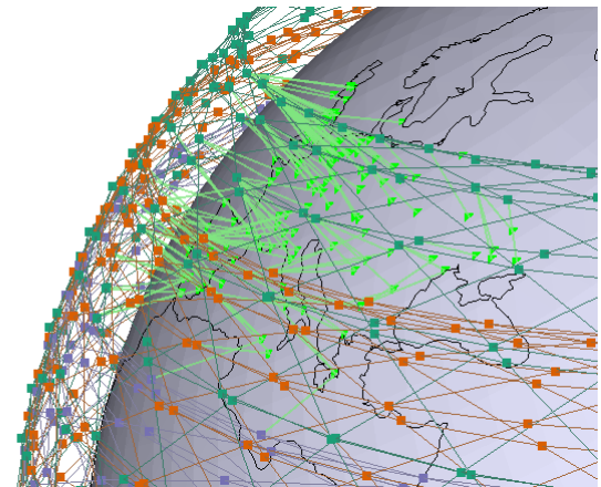
Figure 13: In our experiments, clients in 120 European cities (bright green) access the Kuiper network to interact with the Twissandra web application. The first shell with a 51.9^\circ inclination (turquoise) can be accessed by clients in all of Europe except parts of Scandinavia, which we omit from our experiments. The shell at a 42^\circ inclination (orange) is accessible only in more southern cities, while that at a 33^\circ (purple) is inaccessible to almost all client locations.
